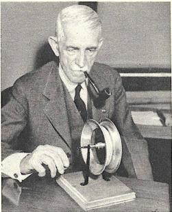
To keep his fly casting lines in good condition, F. L. Scott, of St. Louis, Mo., constructed this novel reel from two pie pans. Reel exposes more line for drying.
