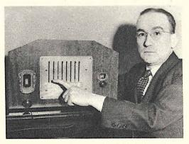
LeRoy L. Leishman, of Los Angeles, Calif., is shown demonstrating his invention which automatically tunes in either television or broadcast station, or both, merely by pressing lever.
