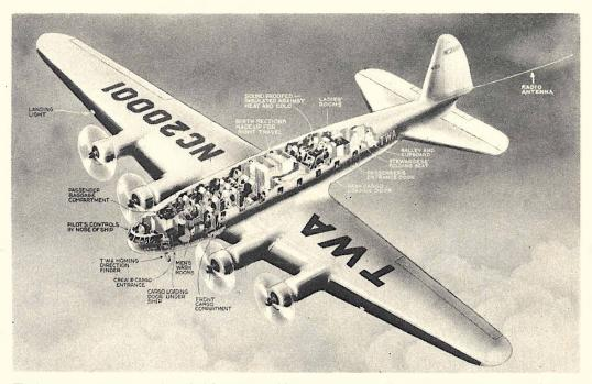
The largest passenger plane in the United States, powered by four 1,205-horsepower engines, has been ordered, and is expocted to be placed in service next spring. Carrying 32 passengers, the monster ship-will be capable of 250-mile-an-hour speed at 20,000-foot altitudes. Cabins are designed for supercharging for high altitude flying. Ship weighs 42,000 pounds.
