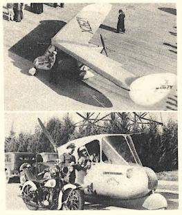
Top---New Arrowbile ready to fly. Below----Wings detached and ready for operation as an automobile. Using a Studebaker engine, the vehicle is capable of a 70-mile-an-hour land speed.
