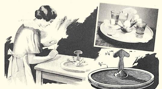
This attractive Hors-d'oeuvre Tray makes an attractive oneevening project for the workshop fan. Constructed from maple plywood and solid stock it requires only a jig saw and lathe for machining. Dimensions of components are shown at right.
