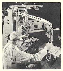
This electric pantograph machine enables the operator to trace the contours of a model with a right hand tool while a left hand tool reproduces the design on a die block.
