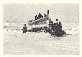
Pushing heavy life boats over sand for launching is eliminated by Netherlands Coast Guard units by using special tractors and trucks to push boats into the surf until they float.
